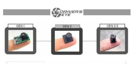
Driver's Eye<sup>™</sup> is the Smallest micro camera in the world For live tv broadcasting (≈1.4gr, 9x9mm)
