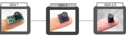
Driver's Eye™ is the smallest micro camera in the world for live TV broadcasting (≈1.4gr, 9x9mm)
